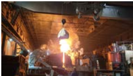
Industrial testing to investigate the use of manufactured bricks from various residual materials in EAF steelmaking.
